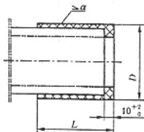
Figure B.2 the layout of taper opening at the end of the pipe
