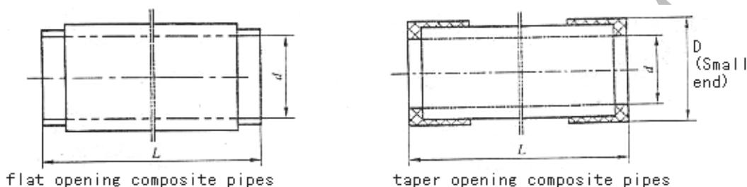
Figure 2 the length of composite pipes
