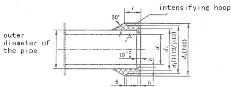
Figure A1 flange connection
