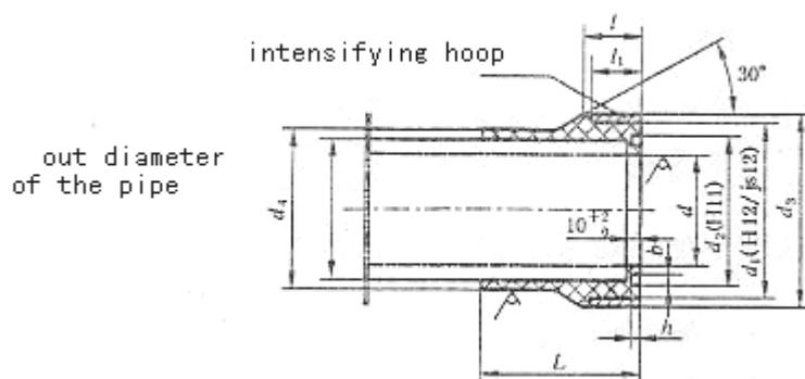
Figure A2 flange connection
