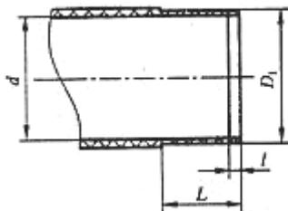
B.1 the outlay of the flat opening at the end of the pipe
